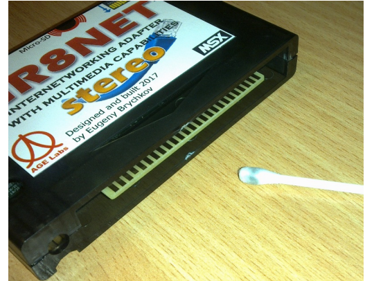
Cotton bud after connector cleaning; dirty edge connector may cause instability in your PC operation using external devices
